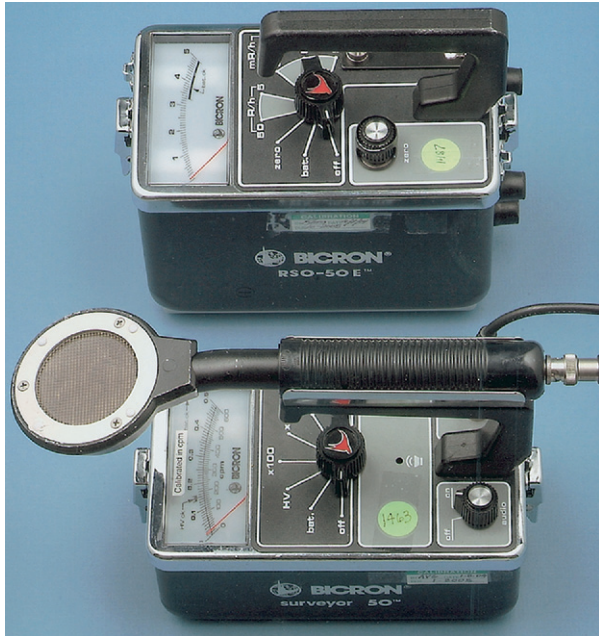
Figure 1. A GM survey meter (below) will detect small amounts of radioactive contamination. It is useful in locating contamination and assessing the effectiveness of decontamination efforts. An ion chamber survey meter (above) will measure the exposure rate from X- and gamma radiation.
